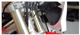
2. Attach X2 to the motorcycle using the rubber mounting straps around the forks.
