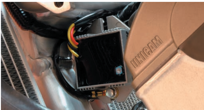
Step 4) Trail Tech regulator/rectifier installed.
