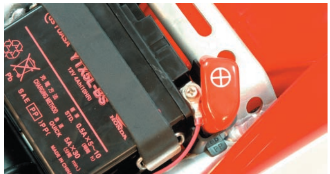
Step 5) Stock light rewired (move from AC to DC.)
